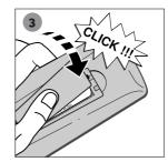
Insert two LR06 or AA batteries in the remote control as shown opposite.
